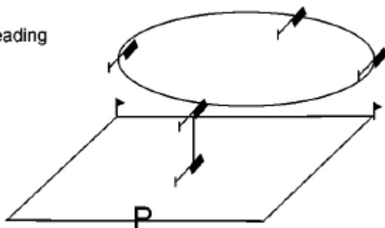
**3. Tail-in Vertical Rectangle.** Model takes off from the central helipad and rises vertically to eye level, pauses, maintaining a constant altitude, heading, and speed, hovers sideways either direction, to the edge of the box, pauses, rises vertically 2m, pauses, hovers sideways over the central helipad to the opposite side of the box, pauses, descends vertically 2m, pauses, hovers back to central helipad, pauses, and descends vertically to the central helipad.
