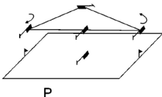
**2. Constant Heading Eight.** Model takes off from the central helipad and rises vertically to eye level, pauses, begins a forward hovering circle, maintaining a constant altitude, heading, and speed, in either direction. The circle passes over
