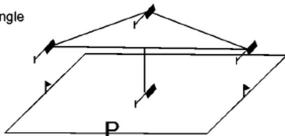
**2. Constant Heading Circle.** Model takes off from the central helipad and rises vertically to eye level, pauses, maintaining constant altitude, heading, and speed, completes a circle to the right or left. The circle passes over the two (2) corner flags opposite the pilot ending over the central helipad, pauses, descends vertically, and lands on the central helipad.
