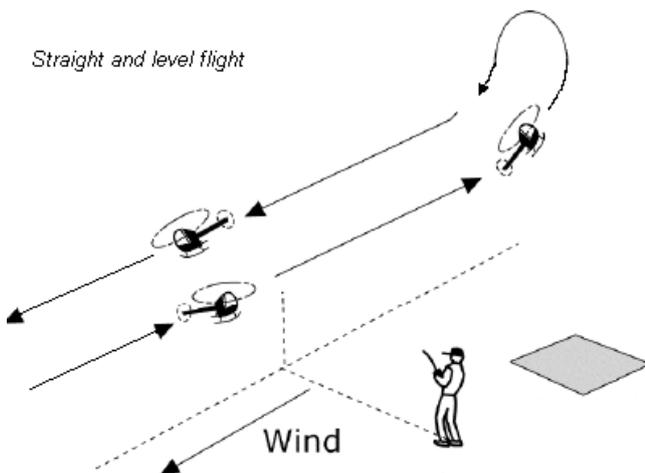
**5. Figure 8.** The model moves away at its chosen height for a distance of about fifteen meters, turn away from the pilot, continue turn through more than 180 deg and bringing the model back across in front of the central helipad, continues at
