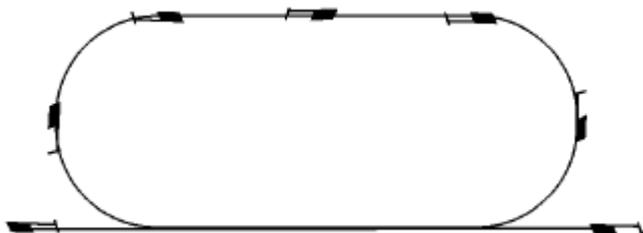
**7. Stall Turn with Half-Roll.** Model flies straight and level for 10m, climbs vertically with a smoothly rounded curve, stops, rotates 180 degrees so the nose is downward, executes half-roll, either direction, and recovers to straight level flight 10m at original altitude. Note: there should be a helicopter length of straight flight between the rotation and the half-roll, and between the half-roll and the recovery. Vertical line should be on the midline.
