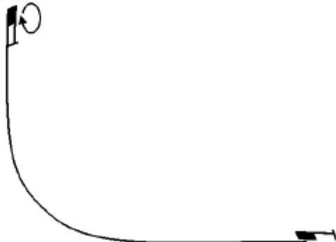
**5. Slow Roll.** Model flies straight and level for a minimum of 10m, rolls through one (1) complete 360 degree revolution maintaining the nose in the direction of flight, flies straight and level for the same duration and at the same altitude as the entry. Manoeuvre is centred with the model inverted at the midline and the roll portion of the manoeuvre should have a duration of 3 seconds minimum.
