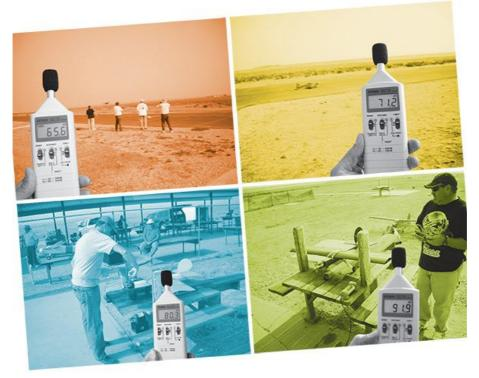
During engine run-up the pilot is exposed to significant short-term noise levels. Although seldom used, hearing protection is a good idea, even with limited exposure. Sound levels at the pilot's position during a flight are typically 75 dBA or less.
