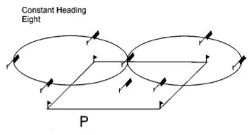
**3. Spike with 90 and 180 Degree Pirouettes.** Model takes off from the central helipad and rises vertically to eye level, pauses, rotates 90 degrees in either direction, pauses, climbs vertically 2m, pauses, rotates 180 degrees in the opposite direction, pauses, descends vertically 2m, pauses, rotates 90 degree in the original direction, pauses, descends vertically to central helipad.
